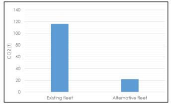
Figure 4: Comparison of CO<sub>2</sub> emissions existing fleet vs. alternative fleet Journal of Applied Engineering Science 15(2017)1, 413
